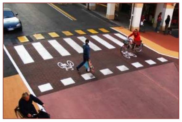
Figure 36: Example of a speed table
