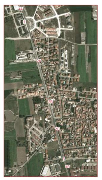
Figure 20: Final proposals - (1-3 mini roundabouts; 2 A-B-C speed tables; 4 A-B measures at the entrance of the town)
