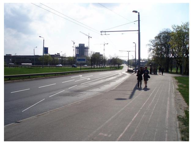
View in the opposite direction. Arrows show in which direction each lane would go. When heavy traffic about 900-1200 vehicles per hour would go straight and 300-400 later turn right.
