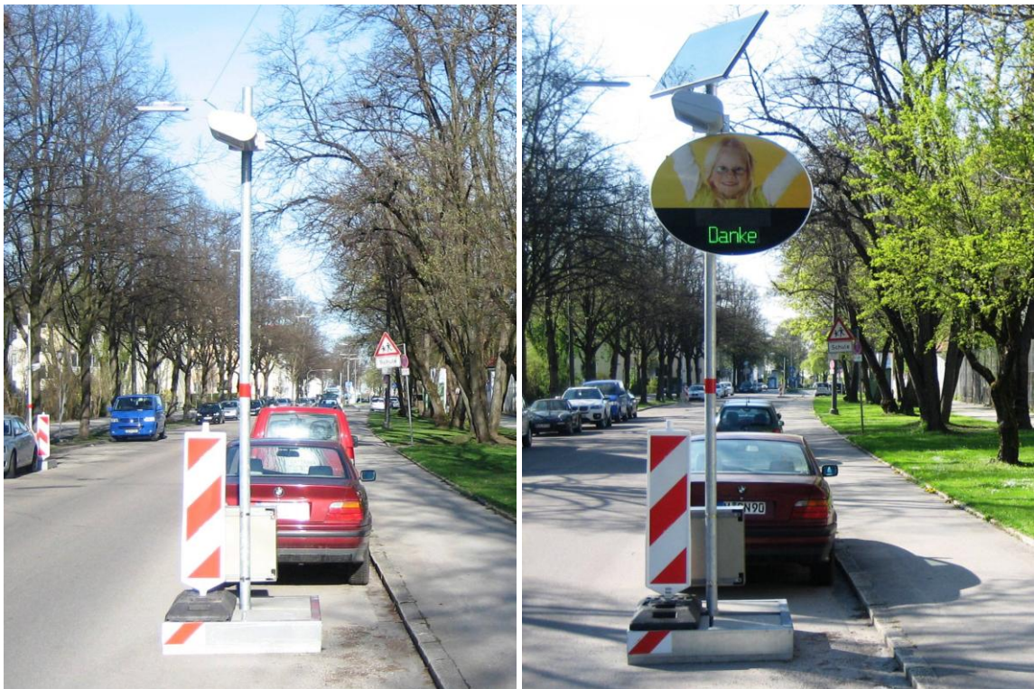
Figure 9 Speed Measurement Detector (left) for the Assessment of the previous Situation and installed Dialog-Display (right). Direction: Herkomerplatz. Spot 3
