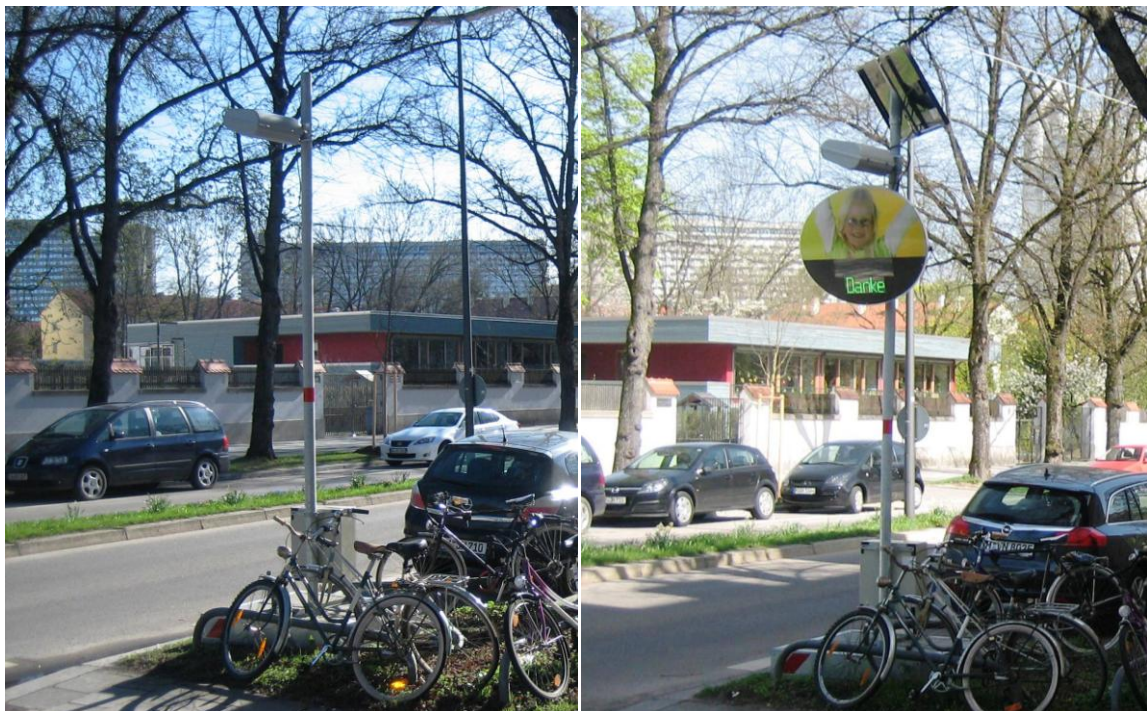
Figure 8 Speed Measurement Detector (left) for the Assessment of the Previous Situation and installed Dialog-Display (right). Direction: Richard-Strauß-Straße. Spot 3
