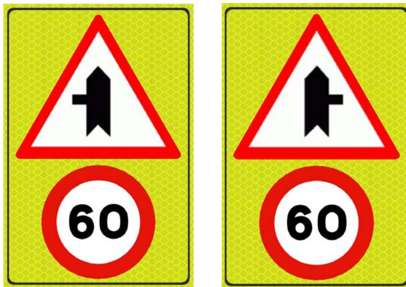
Illustration 19: Fluorescent reflective yellow sheet panels with “dangerous crossing” and “speed limit” signs.
