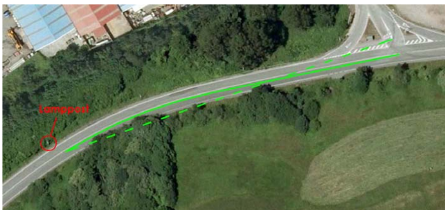
Illustration 18: The crossing distance can be measured using an orthophoto, proving to be 163 m.
