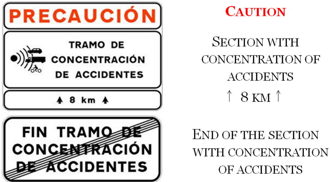
Illustration 52: Signs which are used to signpost the beginning and the end of a stretch of accident concentration.
