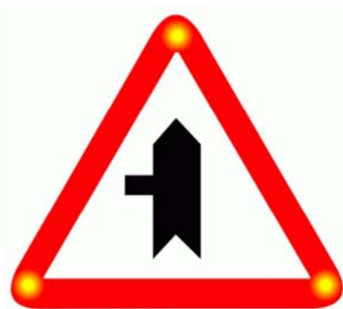
Illustration 59: Representation of the light sign proposed to warn about a dangerous crossing.
