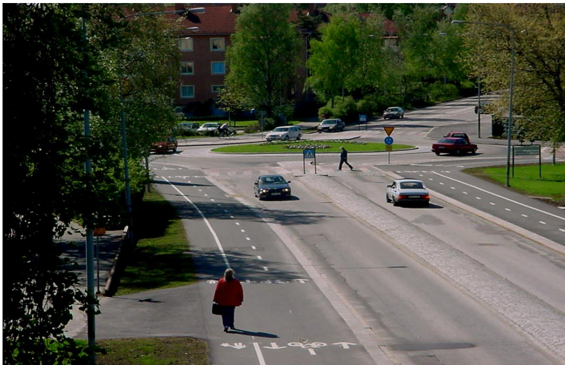
Ideal: Trollhättan, Sweden (separate footway and bicycle lane; safe crossing; traffic calming measures...)
