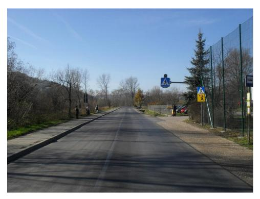
The wide of the road is  $2 \times 3,25$  so it's 6,50 m. On the left there is a pavement 2,20 m wide. On the right is a small bus stop with a lay-by made of gravel.
