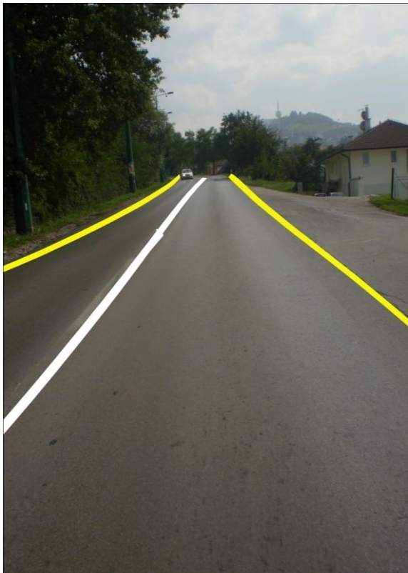
Picture 8.: Proposal to treat high risk site: Pavement road markings and installation horizontal and vertical signs
