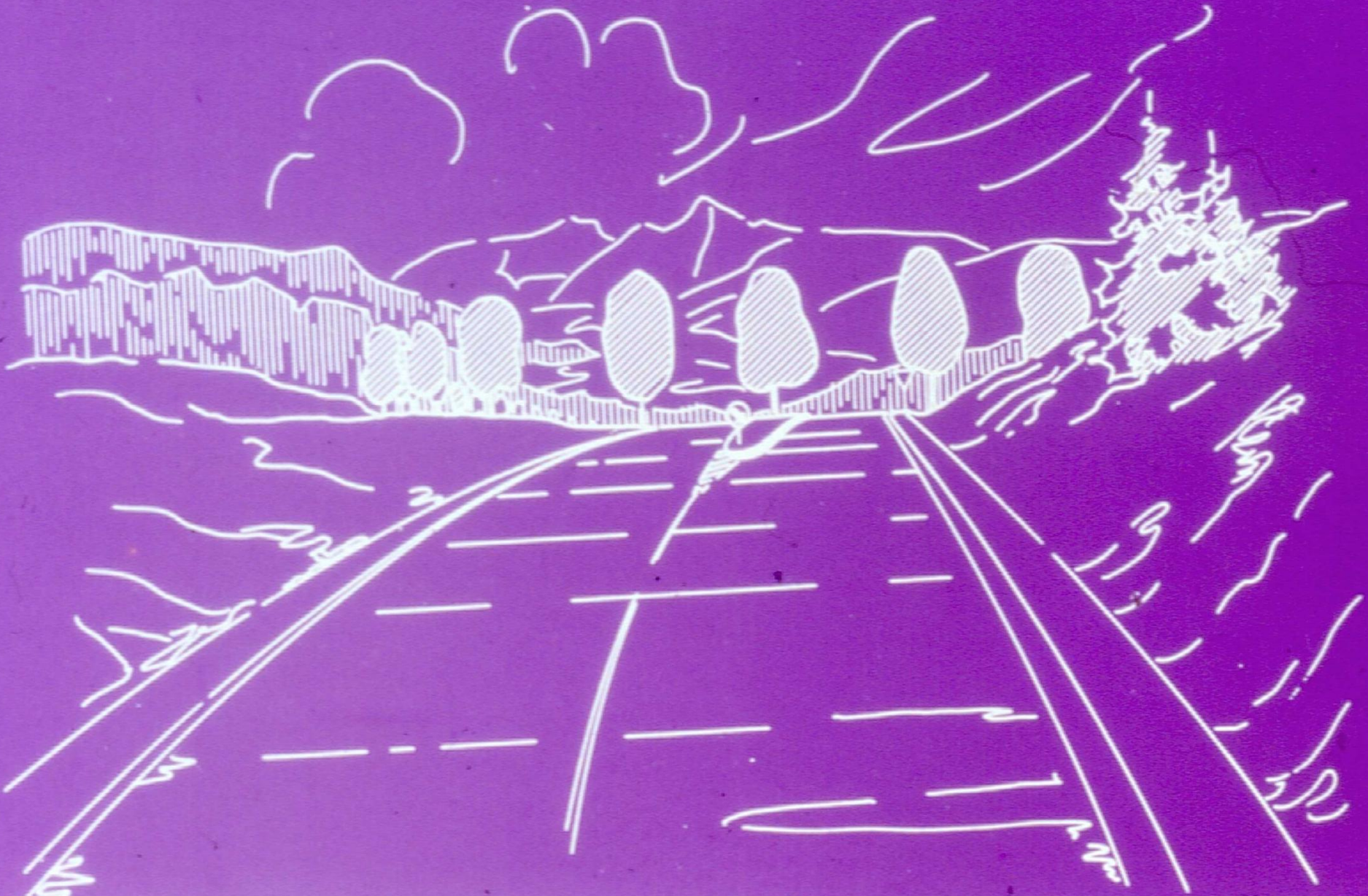
Intersection should be recognizable Combination of crest curve with intersection
