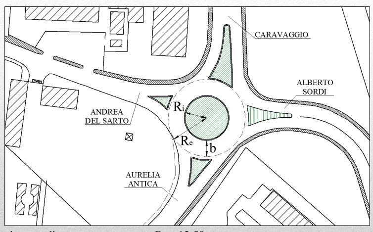
inner radius outer radius circulatory roadway width  $R_i = 12,50 \text{ m}$
